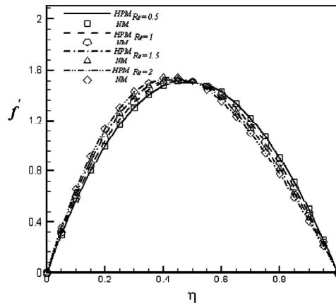
Figure 3: Velocity Component Profile ( $f'$ ) for Variable  $Re$  at  $K_1 = 0.01$
