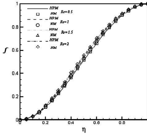
Figure 2: Velocity Component Profile ( $f$ ) for Variable  $Re$  at  $K_1 = 0.01$
