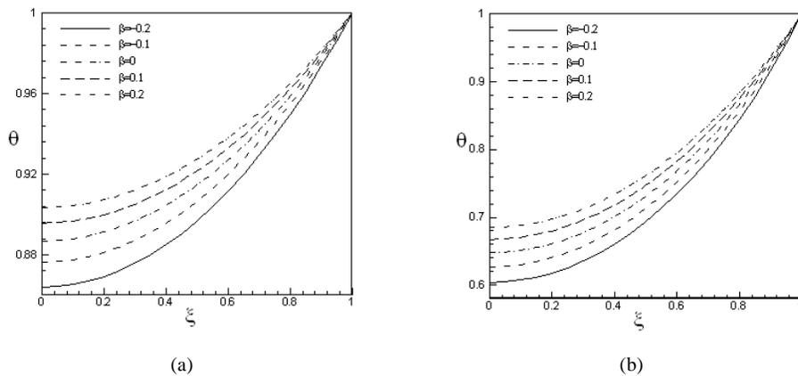
Figure 5: Temperature Distribution in Convective Fins with Variable Thermal Conductivity. (a) When  $\psi = 0.5$ , (b) when  $\psi = 1$ .
