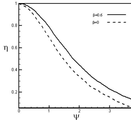
**Figure 6:** Variation of the Fin Efficiency with the Thermo-Geometric Fin Parameter ( $\psi$ ) for Different Values of the Thermal Conductivity Parameter
