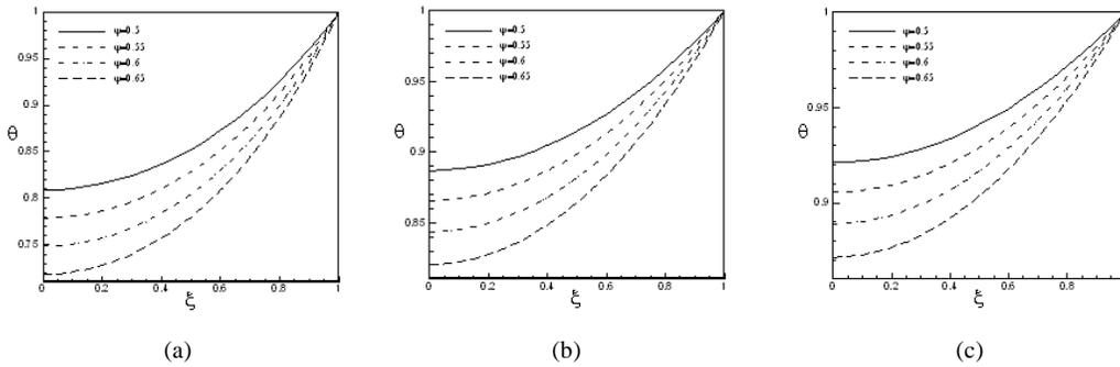
Figure 4: Temperature Distribution in Convective Fins with Variable Thermal Conductivity. For Various  $\psi$  when (a)  $\beta = -0.5$ , (b)  $\beta = 0$  and (c)  $\beta = 0.5$ .
