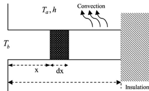
Figure 1: Geometry of a Straight Fin
