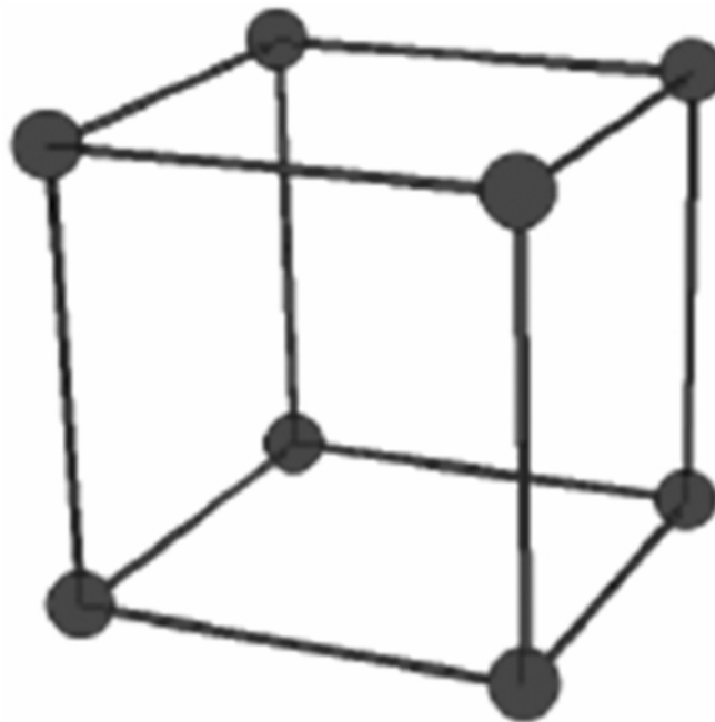
Fig. 13: Platomic Rocksalt Structure as the Structure of \text{NaCl} , this Network can be Represented by the Wells Point Symbol (4^{12}) , and Lies in Space Group (Pm-3m)
