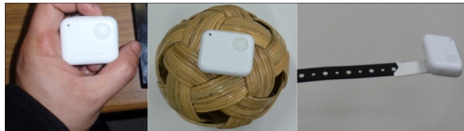
Figure 9. 3D accelerometer sensor attached to hands, ball and stick objects.
