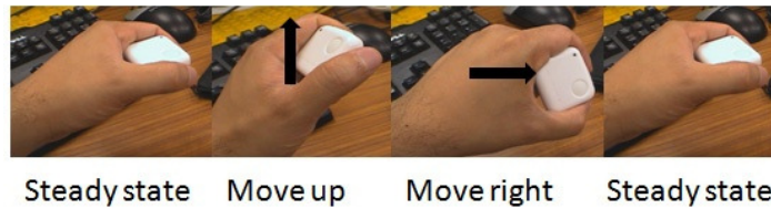
Figure 7. Tilt sequence, building a sequence of tilt movements up, followed by right.
