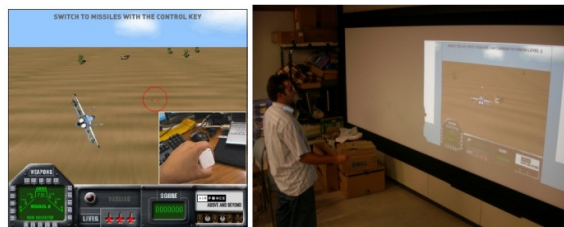
Figure 5. Left: tilting sensor to control flight speed; Right: user interacting with flight simulator.
