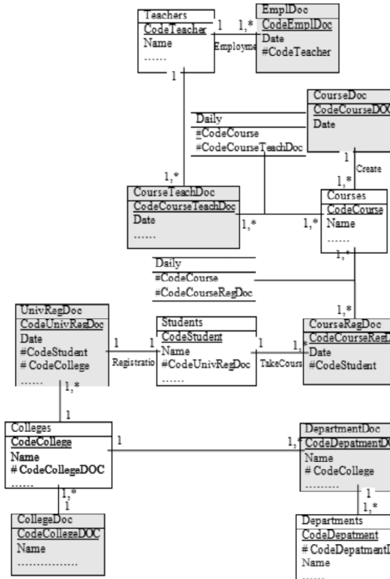
Figure 2: The Association Diagram for the University Database system
