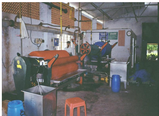
Figure 2 Jigger Type Dyeing
