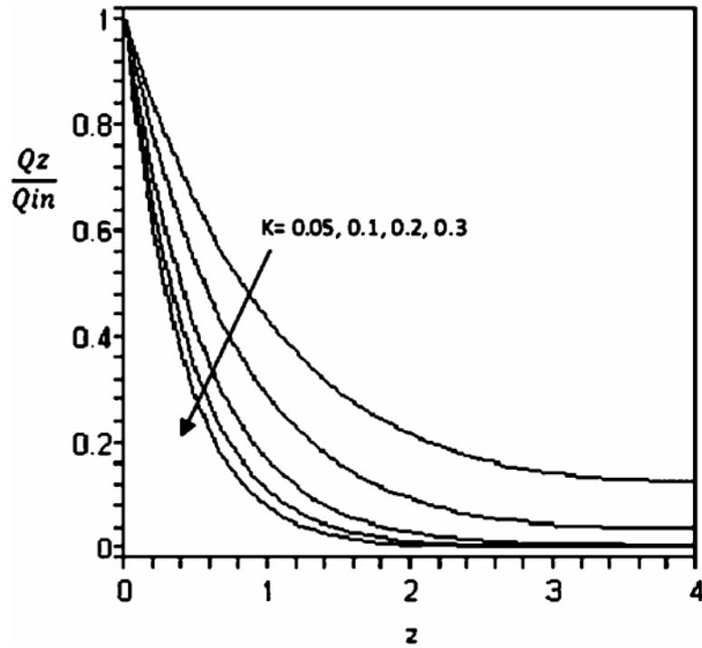
Figure.7: Ratio of Axial Mass Transfer to Entrance Mass Transfer Profile with Respect to  $z$  at Various  $k$
