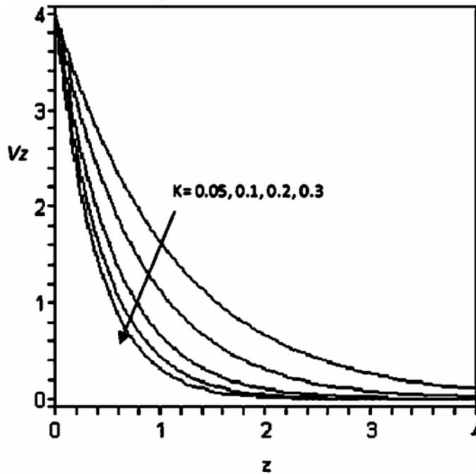
Figure.3: Axial Velocity Profile with Respect to  $z$  at Various  $k$  and  $r = 0.1$
