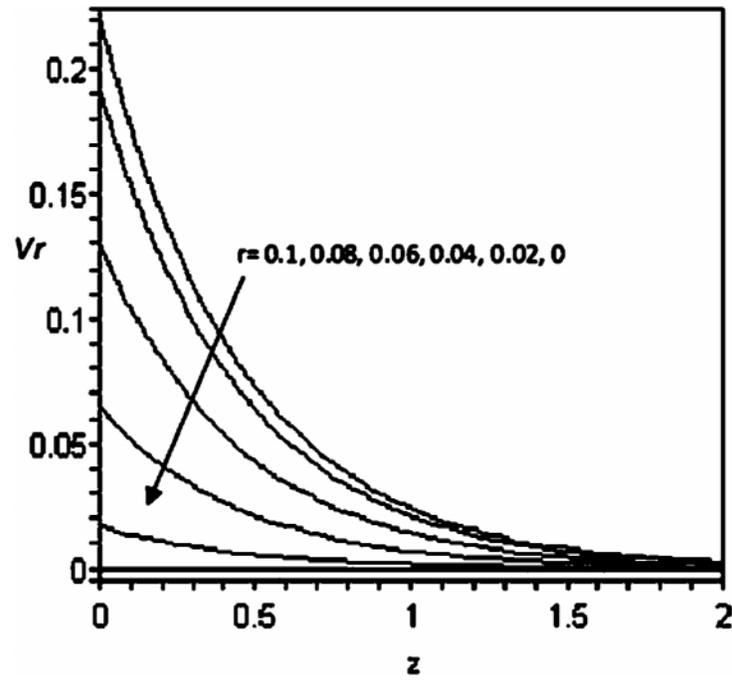
Figure.6: Radial Velocity Profile with Respect to  $z$  at Various  $r$  and  $k = 0.2$
