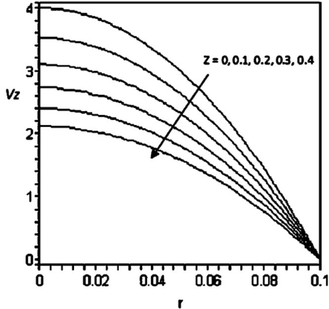
Figure.2: Axial Velocity Profile with Respect to  $r$  at Various  $z$  and  $k = 0.1$
