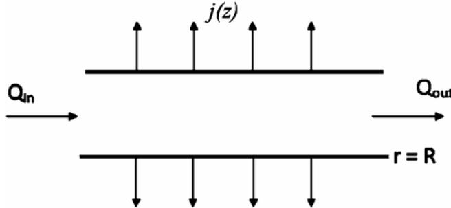
**Figure.1:** Schematic View of a Typical Laminar Flow through a Leaky Tube
